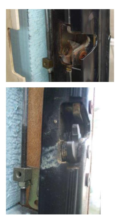
Now put it all back together. Use some contact cement on the gasket at the door corners to glue the gasket back together. You can put the contact cement on before you install the door end and let it dry till it is a bit tacky. Then put the end in place, install the screws, and now press the seal corners together tightly for a few seconds. The contact cement should hold the gasket together almost immediately.
